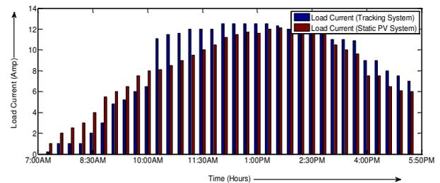
**Figure 5.10** Variation in load current due to one degree of freedom (Y-axis tracking)
