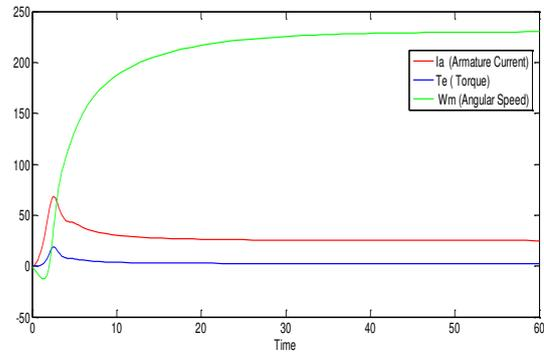
**Figure 4.13** Simulation result of SWDC motor directly connected to PV module
