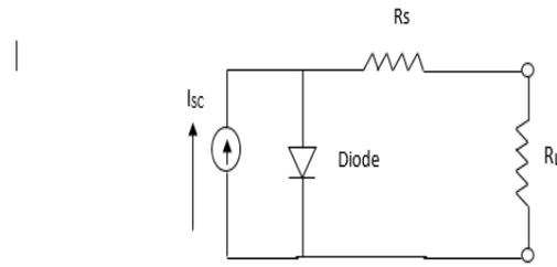
**Figure 3.7:** Equivalent circuit used in the MATLAB simulations
